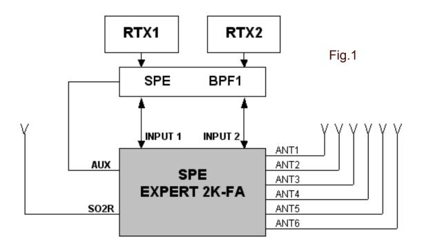
This scheme is suitable for not very sophisticated stations with antennas that are frequently for "two or three bands."
