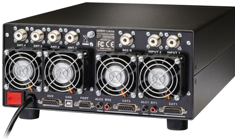
Figure 9 — Rear-panel view of the SPE Expert 1.3K-FA amplifier. The four antenna connectors are at the upper left, while the RF input for two radios and the SO2R connector are at the upper right. Along the bottom are connectors for interfacing two transceivers and USB and serial ports for computer connectivity/remote control.
