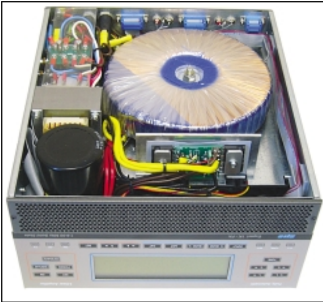
Photo B— The bottom (power supply) portion of the amplifier. Look at that power transformer!
