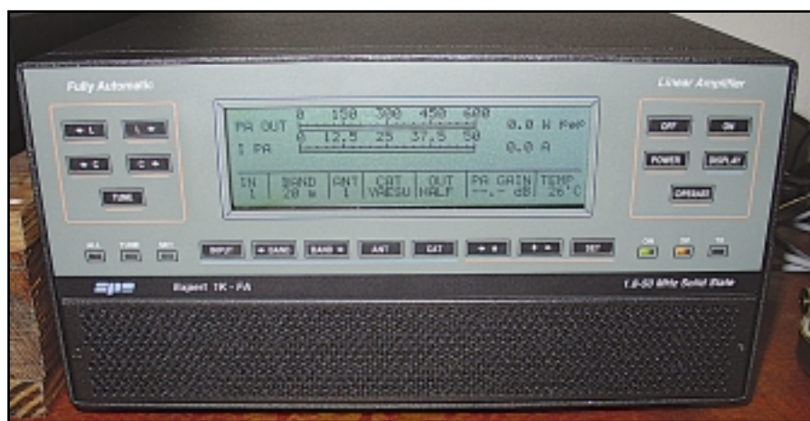
Photo A— The SPE 1K-FA solid-state amplifier puts out 1000 watts on 160–10 meters and 700 watts on 6 meters.
