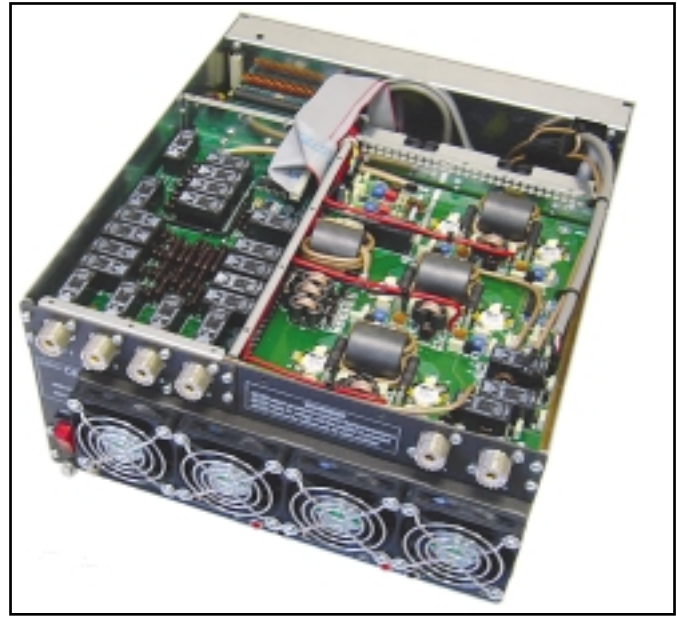
Photo C— RF section of the amplifier with the internal shields removed.
