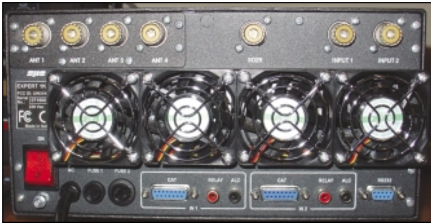
Photo F— Interfaces for transceivers and antennas are well-marked and self-explanatory. Note the SO2R connector.
