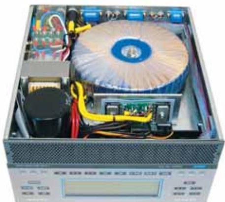
Photo 2: The underside of the linear is dominated by the large toroidal transformer
