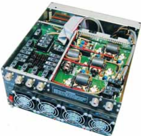
Photo 3: The six MOSFETs on the right are arranged as three push-pull pairs. On the left is the auto ATU section.
