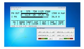
• **REMOTE DOWNLOAD** : Through the "TERM" it is also possible to download the new software releases that are released over time.
